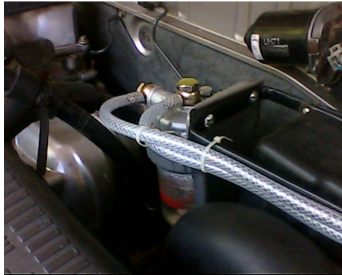
Fig. 4 Bubbler connecting for protection of back fire
